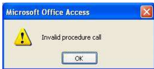
Figure 1. Error message appears as a result of an attempt to calculate the Log(0) value in SQL query
