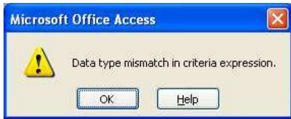
Figure 2. Exception happens when trying to open SQL query (Listing 6), caused by one or more rows in Table 1 containing Null
